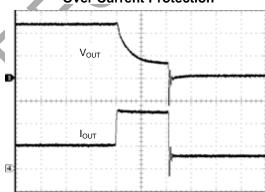
$C_{\text{OUT}}$  = 10 µF,  $C_{\text{IN}}$  = 10 µF,  $I_{\text{OUT}}$  = 2A to 5.6A CH1: V\_{OUT}, 0.5V/Div, DC CH2:  $I_{\text{OUT}}$ , 2A/Div, DC TIME: 0.2ms/Div
