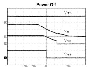
$C_{OUT}$ =10 $\mu$ F,  $C_{IN}$ =10 $\mu$ F,  $R_L$ =0.4 $\Omega$
