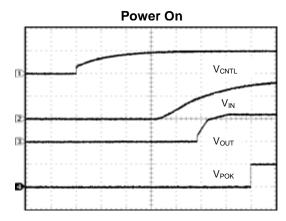
$\begin{array}{l} C_{OUT} \! \! = \! 10 \mu F, \, C_{IN} \! \! = \! 10 \mu F, \, R_L \! \! = \! 0.4 \Omega \\ CH1: \, V_{CNTL}, \, 5 V/Div, \, DC \\ CH2: \, V_{IN}, \, 1 V/Div, \, DC \\ CH3: \, V_{OUT}, \, 1 V/Div, \, DC \\ CH4: \, V_{POK}, \, 5 V/Div, \, DC \\ \end{array}$ TIME: 2ms/Div
