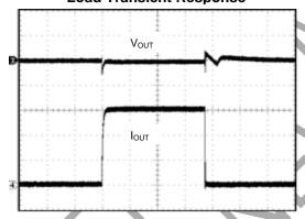
$l_{OUT}$  = 10mA to 3A to10mA (rise / fall time =1µs)  $C_{OUT}$  = 10µF,  $C_{IN}$  = 10µF CH1:  $V_{OUT}$ , 50mV/Div, AC CH2: I<sub>OUT</sub>, 1A/Div, DC TIME: 50µs/Div
