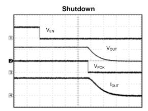
$$\begin{split} &C_{OUT} = 10 \mu F, \ C_{IN} = 10 \mu F, \ R_L = 0.4 \Omega \\ &CH1: \ V_{EN}, \ 5 V/Div, \ DC \\ &CH2: \ V_{OUT}, \ 1 V/Div, \ DC \\ &CH3: \ V_{POK}, \ 5 V/Div, \ DC \\ &CH4: \ I_{OUT}, \ 2 A/Div, \ DC \\ &TIME: \ 4 \mu s/Div \end{split}$$
