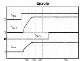
$$\begin{split} &C_{OUT} = 10 \mu F, \ C_{IN} = 10 \mu F, \ R_L = 0.4 \Omega \\ &CH1: \ V_{EN}, \ 5 V/Div, \ DC \\ &CH2: \ V_{OUT}, \ 1 V/Div, \ DC \\ &CH3: \ V_{POK}, \ 5 V/Div, \ DC \\ &CH4: \ I_{OUT}, \ 2 A/Div, \ DC \\ &TIME: \ 1 ms/Div \end{split}$$
