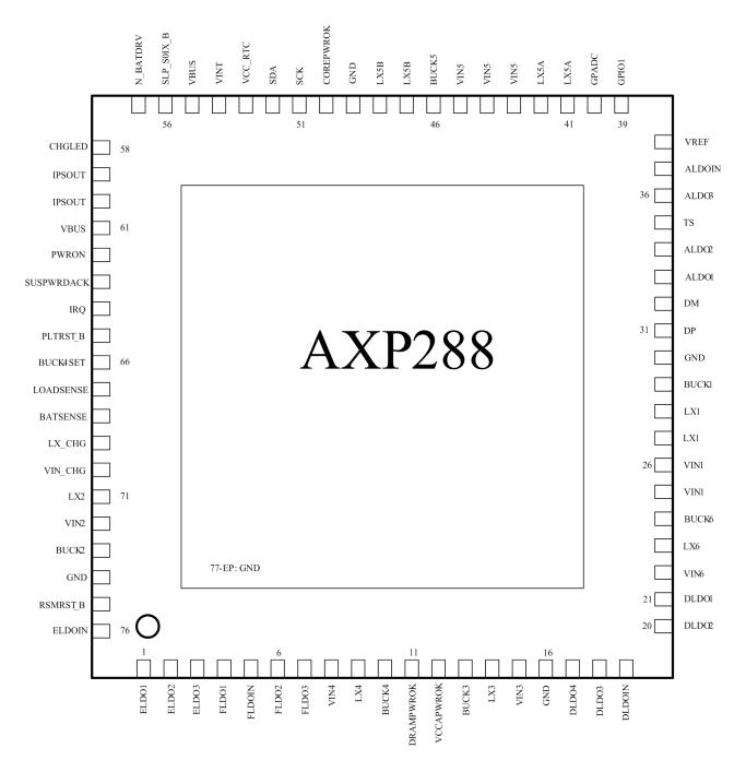
Figure 2. AXP288 Pin Configuration
