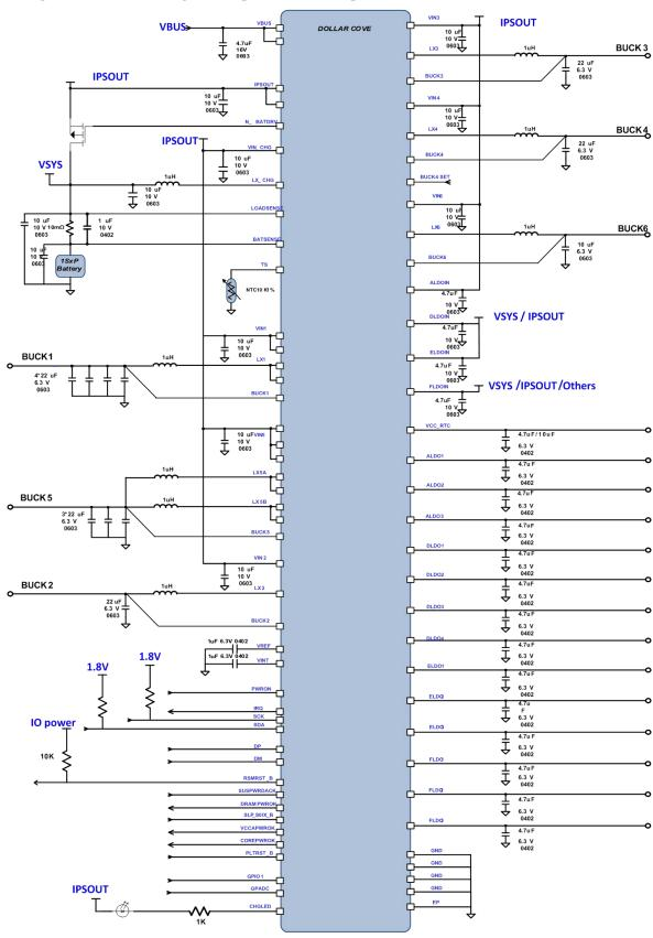
**Figure 1. Typical Application Circuit**
