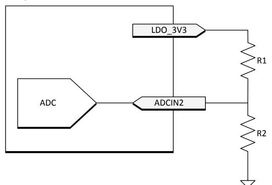
Figure 8-29. I<sup>2</sup>C Address Divider
