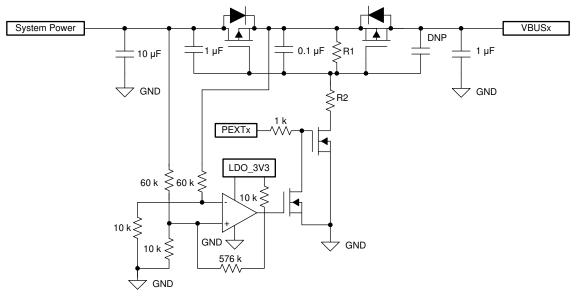
Figure 9-1. Recommended Sink Power Path
