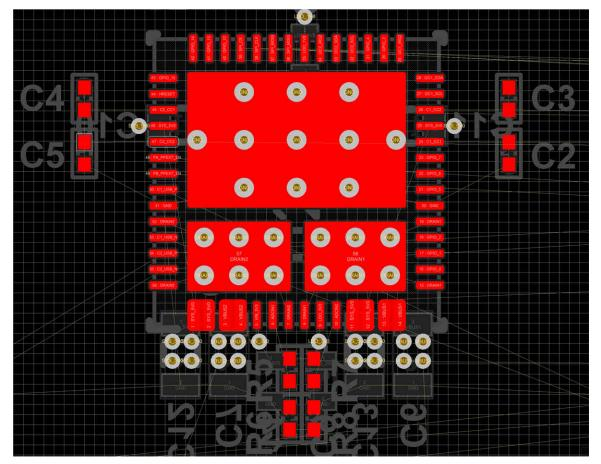
Figure 11-12. CC and ADCIN1/2 Component Placements
