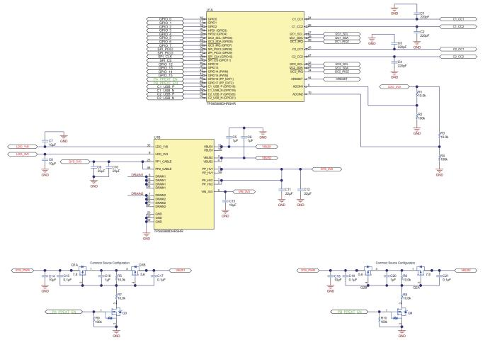
Figure 11-1. Layout Example Device Schematic
