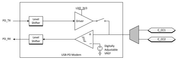
Figure 8-5. USB-PD BMC TX/Rx Block Diagram
