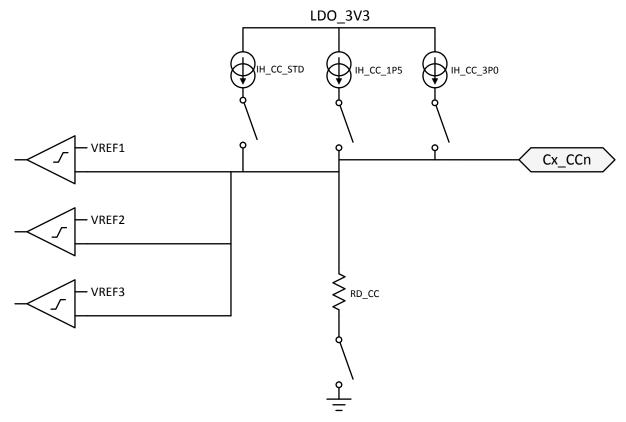
Figure 8-14. Plug and Orientation Detection Block
