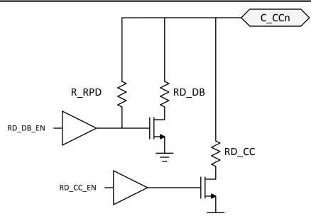
Figure 8-16. Dead Battery Pull-Down Resistor
