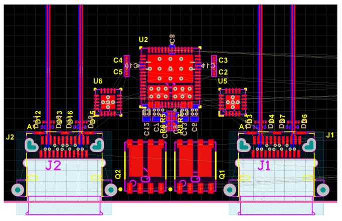
Figure 11-13. Protection Placement
