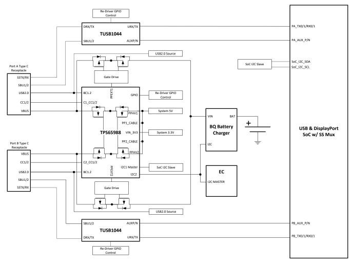
Figure 9-9. TPS65988DJ and SoC I2C with Re-Driver GPIO
