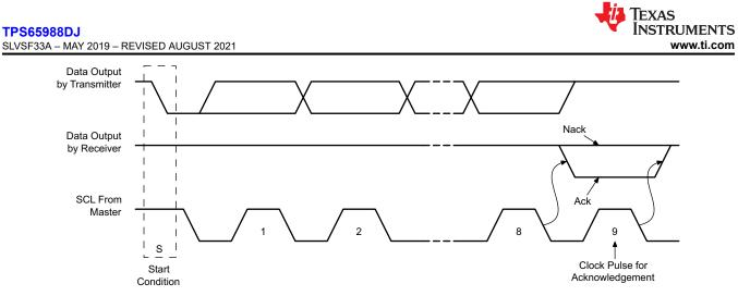
Figure 8-25. I<sup>2</sup>C Acknowledgment
