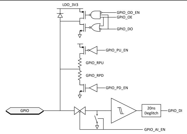
Figure 8-19. General GPIO Buffer
