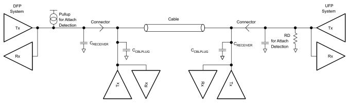
Figure 8-8. Example USB-PD Multi-Drop Configuration
