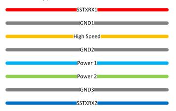
Figure 11-3. 8 Layer Board Stack Up
