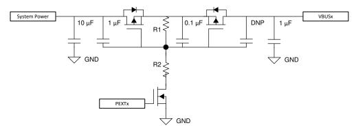
Figure 9-2. Simple Sink Power Path
