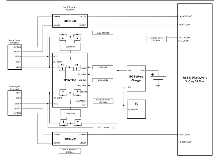
Figure 9-10. TPS65988DJ, SoC and Redriver I2C
