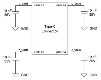
Figure 9-3. Type-C Connector VBUS Capacitors
