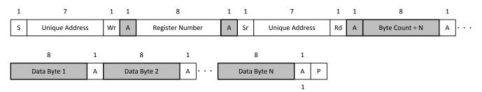
Figure 8-27. I<sup>2</sup>C Unique Address Read Register Protocol
