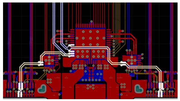
Figure 11-17. Complete USB2 Routing
