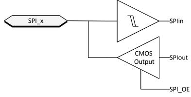
Figure 8-21. SPI Buffer
