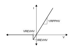
Figure 8-11. Comparator Mode (Source) Internal HV Switch I-V Curve
