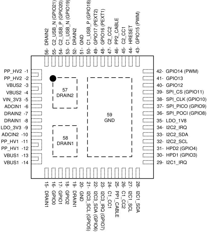
Figure 5-1. RSH Package 56-Pin QFN Top View
