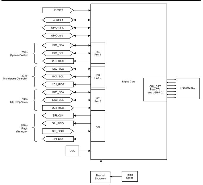
Figure 8-22. Digital Core Block Diagram
