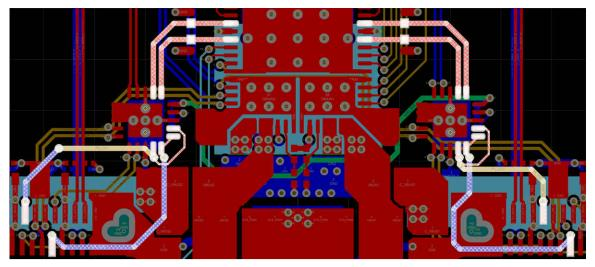
Figure 11-14. Complete CC Routing
