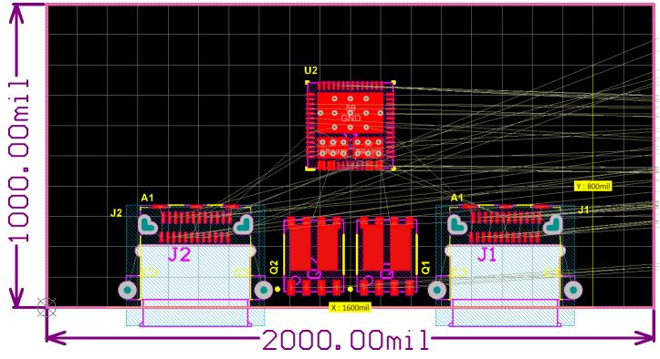
Figure 11-5. High Level Placement
