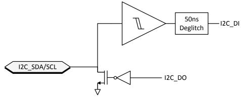
Figure 8-20. I<sup>2</sup>C Buffer
