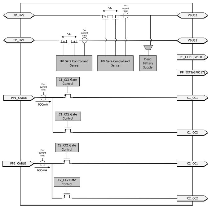
Figure 8-10. Port Power Switches
