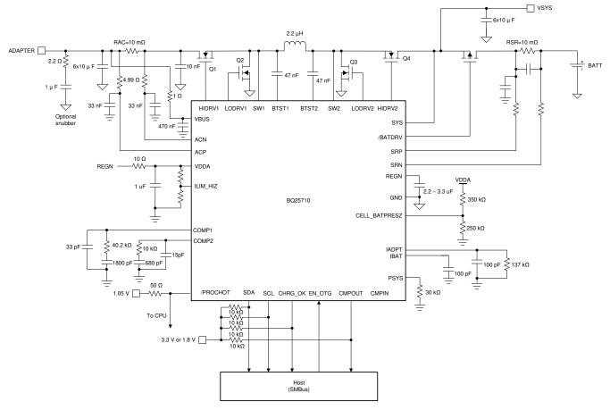
Figure 10-1. Application Diagram
